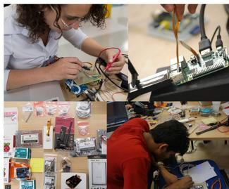
Assembly of 'fast prototyping' electronics components to mobile tracking, communication and demarcation system for demining dogs
